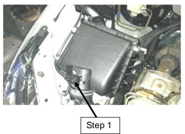
Disconnect the harness connectors from the air flow sensor and unclip the harness from the air box lid. Then undo the hose clamp and remove the engine intake hose from the air box.
