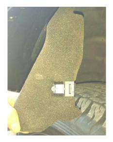
12. Remove and retain the screws that secure the right hand side mud flap. Remove and retain the mud flap
