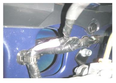
19. From inside the guard, unclip the wire harness from the vehicle and move it out of the way to ensure clearance when drilling in step 20.
