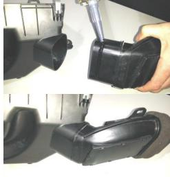
11. Run a bead of neutral cure silicone around the end of the original air box adaptor tube that connects to the air box and refit it back into position ensuring it clips securely. Set aside for fitment later.
