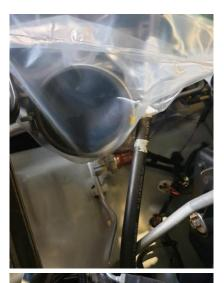
2. Cover the engine intake pipe with a clean plastic bag or similar so no foreign matter can enter the engine.
