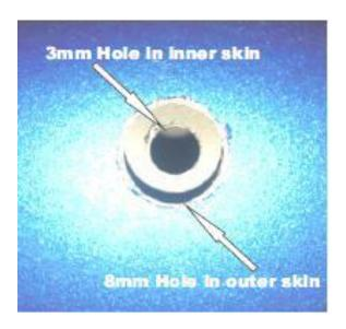
31. Centre-punch the holes marked, then drill 3mm pilot holes at the positions, then drill two 8mm holes.
