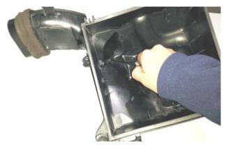
7. Remove the air box adaptor tube from the base of the air box by releasing the clips with a flat head screwdriver as shown.
