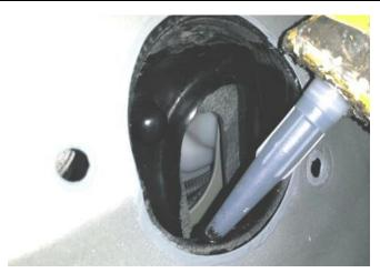
41. Through the 98mm hole in the guard, apply a bead of neutral clear silicone to the inside surface if the intermediate tube at the snorkel end.
