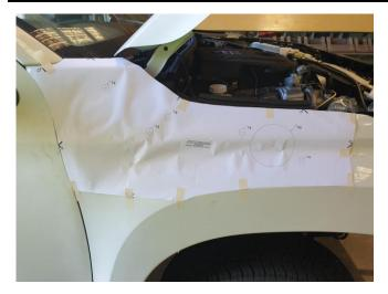
15. Cut the outer guard template and carefully align with the top and rear outer edges of the right hand guard. Tape it in place.
