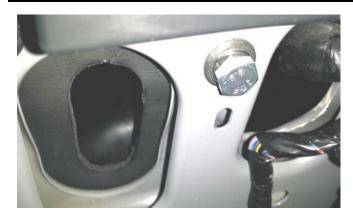
27. Place the intermediate tube in position under the guard and secure it with M8 x 1.25 x 35mm hex bolt (1), M8 spring washer (1) and M8 x Ø19mm flat washer (1)
