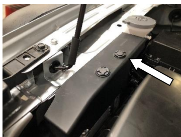
Re - Install Cover
