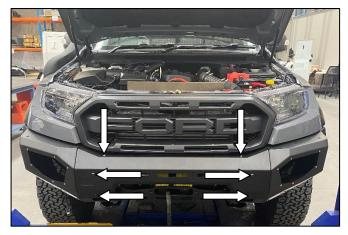
58. With the assistance of another person, carefully lift the bar assembly into position on the "Bar Mounts", then loosely secure it in place, using M10 x 1.5 x 25mm Button Head Bolt (6), M10 x Ø20mm x 1.8mm Flat Washer (6) & M10 x 1.5 Flange Nut (6) at the indicated locations.
