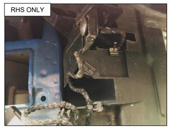
21. Clip the FM antenna cable to the plastic airdam as shown.
