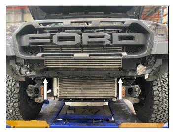
25. Attach the fog light harness to the radiator support panel using zip ties.
