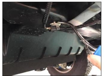
10. Using the trim removal tool, remove the FM antenna clip and connectors from the bumper support beam.
