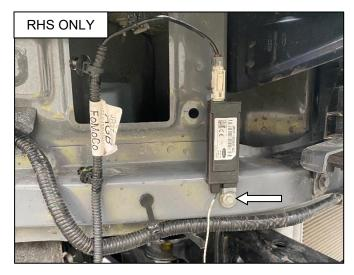
20. Fit the FM antenna box to the right hand side of the radiator support panel using the fastener retained in Step 15 as shown.
