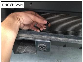
12. Remove and discard the round plastic clip that was securing the lower airdam to the bumper mount.
