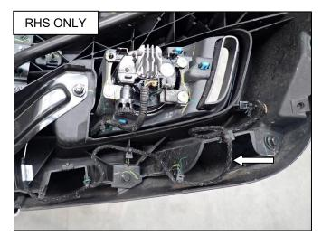
16. Pry the clips away from the bumper that secure the FM antenna harness and cable.
