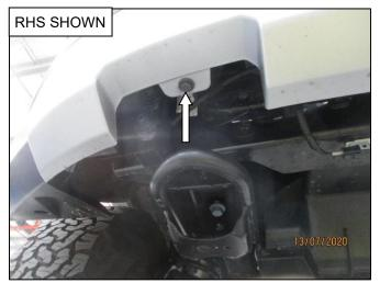
7. Remove and discard the two hex head bolts securing the lower section of the bumper to the vehicle.
