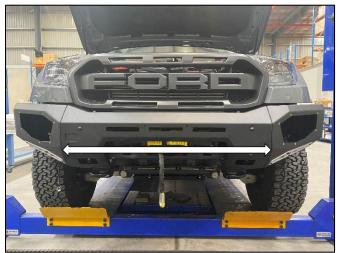
59. Align the bar horizontally across the front of the vehicle and then tighten the fasteners installed in Step 58 to the specific torque settings listed on Page 6.
