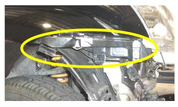
7. Remove & discard both of the plastic bumper return support brackets from the vehicle (RHS shown).
