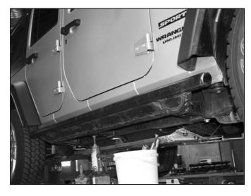
16. Align the Rock Crawler Rails to the vehicle, confirming that the height & angle is suitable, then tighten the installed fasteners to the appropriate torque settings & ensure that as a results of fitting the product, no vehicle components are crushed or will chafe.
