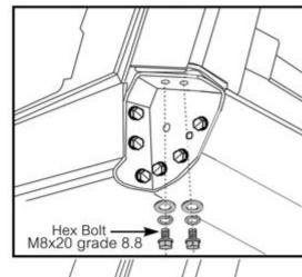
Note: Pre-assemble fasteners by hand then tighten by tool
