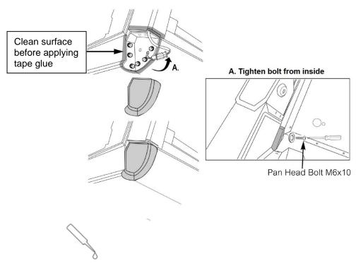
Recommend using Silicone on front corner covers to ensure canopy is fully waterproof
