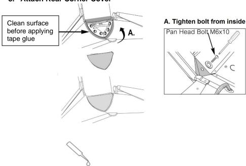
Recommend using Silicone on rear corner covers to ensure canopy is fully waterproof
