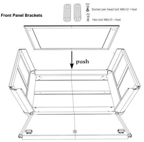
Note: Pre-assemble fasteners by hand then tighten by tool
